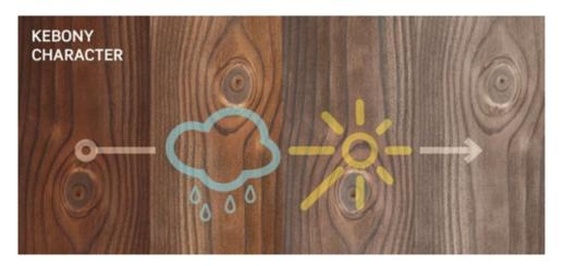
Kebony Character products are produced from FSC®-certified Pinus Sylvestris and contain knots and untreated heartwood. They should not be further machined or split as untreated heartwood will be exposed. Kebony Character products can be cross-cut to length. Exposed end grain after cross-cutting must be treated with a wood preservative.
